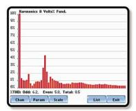
can cause small, almost imperceptible variations in performance that aggregate to effect significant long-term damage. Current harmonics generated by a source can pollute the entire power system without being effected itself. The PowerXplorer captures detailed harmonics, interharmonics and subharmonics to effectively trouble-shoot the complex problems caused by these events.
